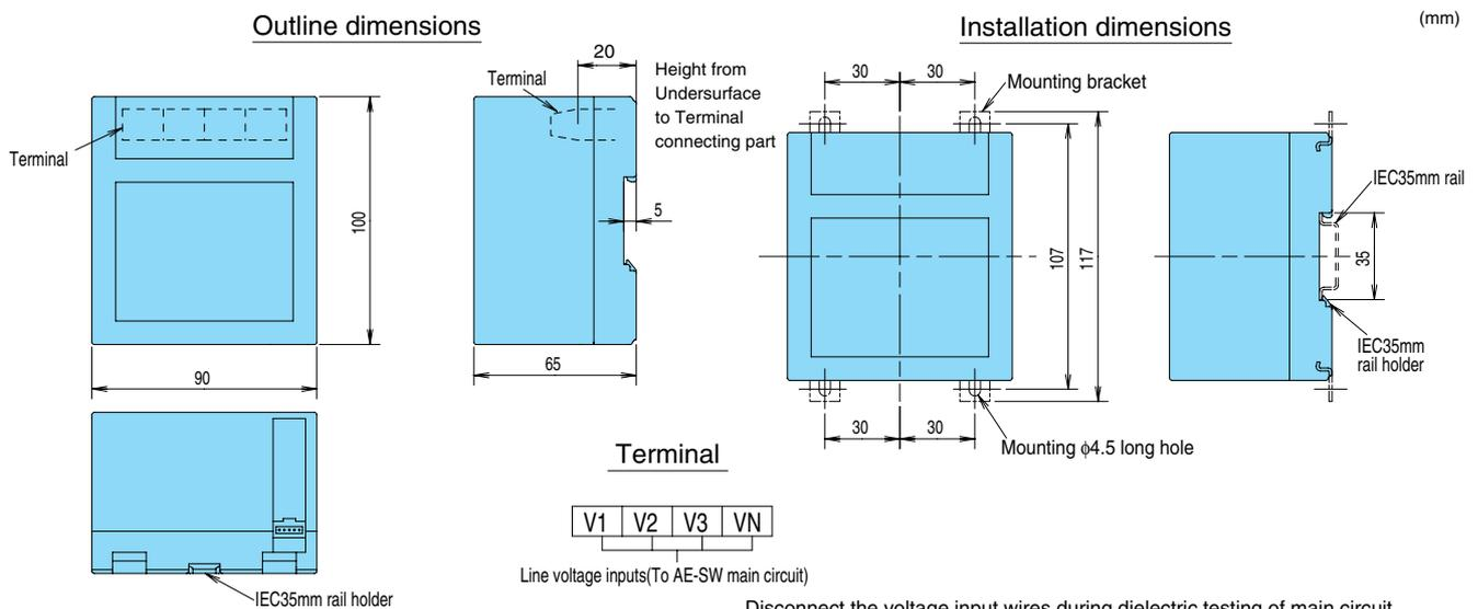
Disconnect the voltage input wires during dielectric testing of main circuit.
