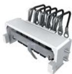
When moving the breaker from the connected to the test positions, this contact is used to short circuit auxiliary switch (AXb), thus maintaining the correct sequence of operation of the external control circuit. When ordering, SBC with the same number of contacts as auxiliary switches (AXb) will be provided.
