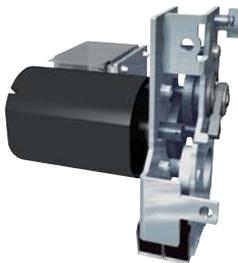
The closing spring is charged by an electric motor. When the breaker is closed, the spring is charged automatically (ON-charge method). The closing coil (CC) is required to remotely close the breaker, and the shunt trip device is required to remotely open the breaker.
