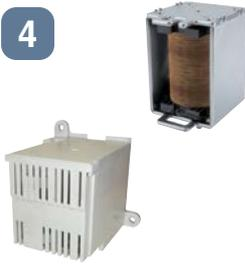
This is the device that automatically trips the breaker when the circuit voltage drops below the nominal voltage, and comprises UVT coil and UVT controller. There are 3 kinds of tripping time, INST, 0.5s and 3.0s. A trip terminal for forced OFF function is included as standard equipment.
