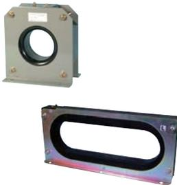
This option is used to detect several amperes of earth leakage when used in combination with an electronic trip relay that has the earth leakage tripping (ER) option. Two methods are available. The first is where the all load conductors pass through the ZCT. The other method uses a smaller ZCT through which the supply transformer's ground wire passes through to the earth.
