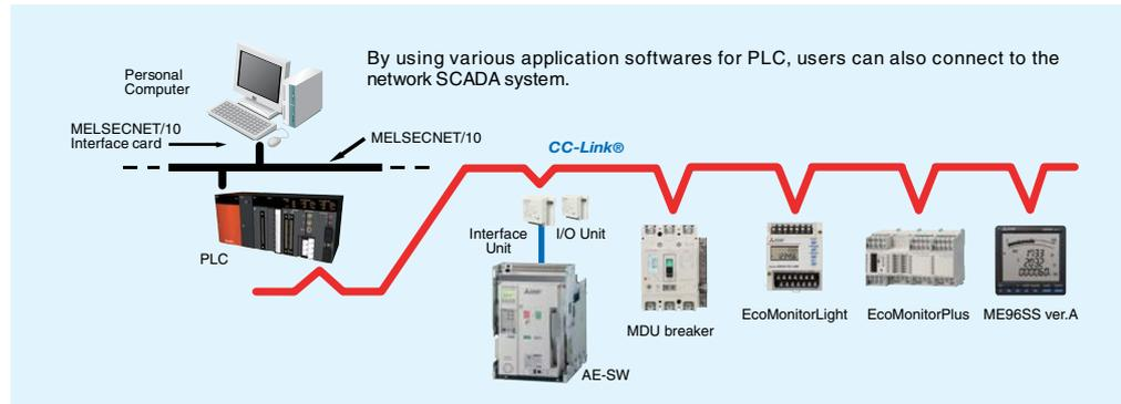
The length of the cable for interface unit is 2m.
