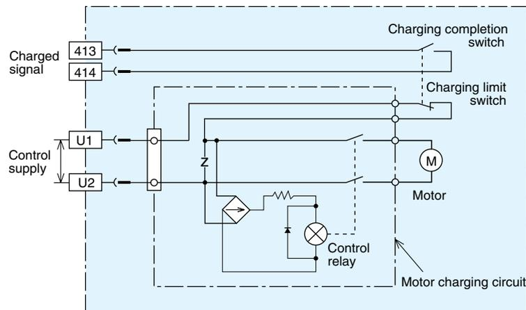
For 24V DC and 48V DC, the Diode rectifier is not included.
