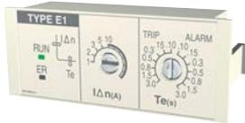
By combining the ETR with earth leakage protection (ER) and External ZCT, earth leakage protection is possible. Earth leakage protection, earth leakage tripping and earth leakage alarm can be selected. Control supply is necessary for this function.
