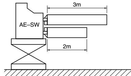
\*1 The temperature rise of rated current 3200A conforms to the requirement of IEC 60947-1 for the connecting conductor size of a rated current 3150A. In case of more than 3200A, conductor sizes are not defined in IEC 60947-1.
