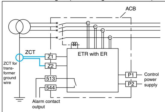
Earth leakage protection characteristics
