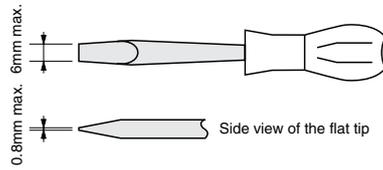
2 Insert the flat tipped screwdriver into the opening of the ETR cover. Then, lightly turn the screwdriver to the upside as shown in the left figure, and the ETR cover will open.
