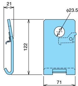
**Fixed type AE400-SW, AE500-SW, AE630-SW**
