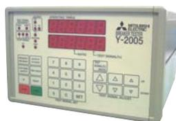
The electronic trip relay can be checked by this field test device when the breaker is at the test position or the disconnect position. The breaker will trip when tested with this device.
