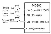
As shown in the preceding figure, if SB1 is ON, the AC drive instructs forward rotation when SB2 is pressed to be ON and instructs reverse rotation when SB3 is pressed to be ON. The AC drive stops immediately after SB1 becomes OFF. During normal startup and running, SB1 must remain ON. The AC drive's running state is determined by the final actions on SB1, SB2 and SB3.
