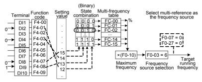
In the preceding figure, DI7, DI4, DI8, and DI2 are used as the multi-frequency input terminals, each of which has a bit value. The state combinations of these terminals correspond to multiple frequencies, When (DI7, DI4, DI8, DI2) = (0, 0, 1, 0), the state combination value is 2, corresponding to the value set in FC-02. The target running frequency is automatically calculated by FC-02 x F0-10.
