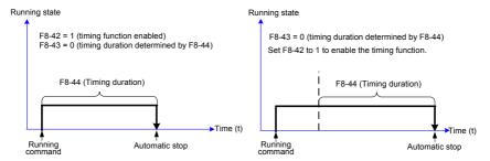
You can set the timing duration by means of analog input (such as potentiometer signal). For details, see the description of F8-43.
