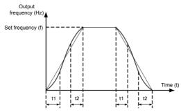
Figure 6-13 S-curve acceleration/deceleration B
