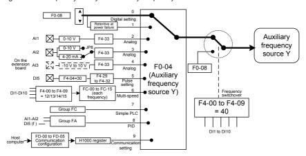
The relationship between the target running frequency and the main frequency source and auxiliary frequency source is set in F0-07, as follows:
