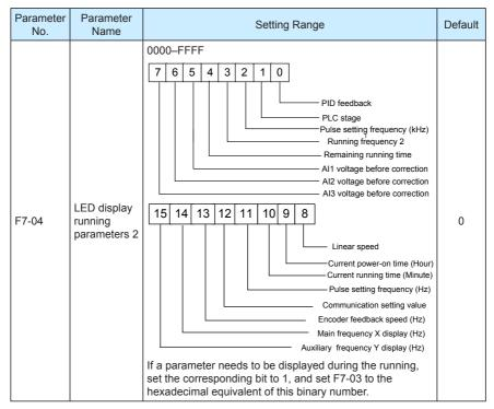
These two parameters are used to set the parameters that can be viewed when the AC drive is in the running state. You can view a maximum of 32 running state parameters that are displayed from the lowest bit of F7-03.
