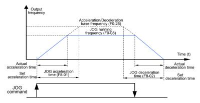
Parameter Setting and Operation of JOG Running in Operation Panel Control
