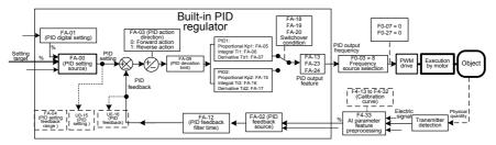
When PID frequency closed-loop control is implemented, F0-03 (Main frequency source X selection) must be set to 8 (PID). The PID-related parameters are set in group FA, as shown in Figure 4-23.
