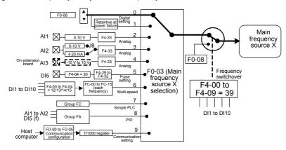
According to the preceding figure, the running frequency of the AC drive can be set by means of parameters, manual adjustment, analog input, multi-speed terminal, external feedback signal, internal PID regulator, or the host computer.
