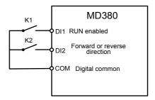
As shown in the preceding figure, if K1 is ON, the AC drive instructs forward rotation when K2 is OFF, and instructs reverse rotation when K2 is ON. If K1 is OFF, the AC drive stops.
