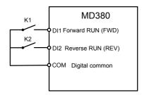
As shown in the preceding figure, when only K1 is ON, the AC drive instructs forward rotation. When only K2 is ON, the AC drive instructs reverse rotation. When K1 and K2 are ON or OFF simultaneously, the AC drive stops.
