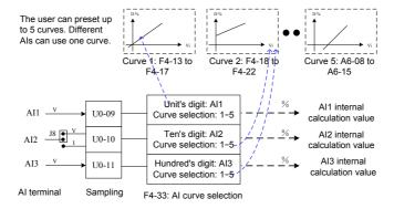
The sampling of AI terminals can be queried in U0-09 to U0-11. The calculation value is for internal subsequent calculation and cannot be directly read by the user.
