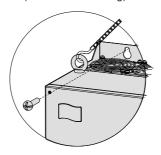
4) Embedded installation of the MD380 (sheet metal housing)
