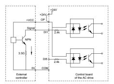
This is the most commonly used wiring mode. To apply external power supply, remove jumpers between +24 V and OP and between COM and CME, and connect the positive pole of external power supply to OP and negative pole to CME.
