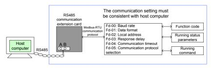
The MD380 arranges the parameters, running state parameters and running commands in the "register parameter address" mode. The host computer can define the protocol of communication data interaction.
