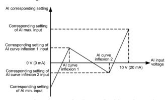
When setting curve 4 and curve 5, note that the curve's minimum input voltage, inflexion 1 voltage, inflexion 2 voltage and maximum voltage must be in increment order.
