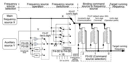
The operation between the main frequency source and the auxiliary frequency source can be used for closed-loop speed control. For example, using the main frequency source for setting the required frequency and the auxiliary frequency source for automatic adjustment, in conjunction with switchover performed by the external DI terminal signal, the required closed-loop control can be implemented.
