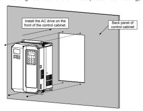
Figure 3-8 Hoisting the MD380 (sheet metal housing)
