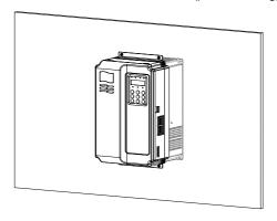
Wall-mounting installation of the MD380 (sheet metal housing)
