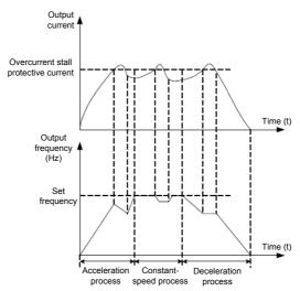
Figure 6-25 Diagram of the overcurrent stall protection function
