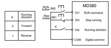
As shown in the preceding figure, if SB1 is ON, the AC drive starts running when SB2 is pressed to be ON; the AC drive instructs forward rotation when K is OFF and instructs reverse rotation when K is ON. The AC drive stops immediately after SB1 becomes OFF. During normal startup and running, SB1 must remain ON. The AC drive's running state is determined by the final actions of SB1, SB2 and K.
