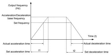
The MD380 provides totally four groups of acceleration/deceleration time for selection. You can perform switchover by using a DI terminal.
