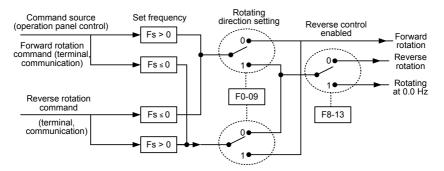
If the command source is terminal control and reverse rotation is required, use the default value 0 of F8-13 to enable reverse control.
